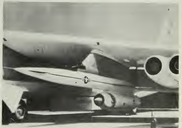
HOUND DOG—USAF's new air-to-ground missile rests in place under wing of B-52 for transportation to target.
